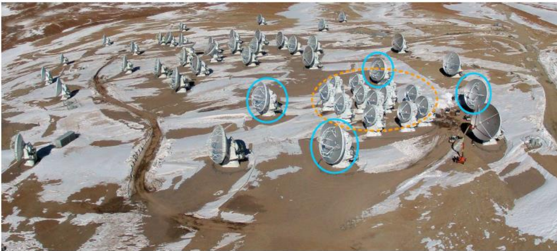
Figure 2.1: The ALMA 12-m Array in its compact configuration (left hand side of the image). The ACA 7-m Array with all 7-m antennas (dashed orange circles) and four single-dish 12-m antennas in the TP Array (blue circles) are distributed in the right hand side of the image. A few unoccupied stations can be seen, to which antennas of the 12-m Array can be moved by the transporter as the array is being reconfigured. At its most extended configuration, antennas in the 12-m Array will be about 16 km apart.
