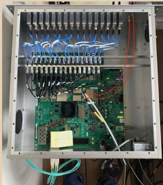
with housing and 16 balun boards
