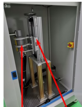
X-ray generator Motion adjusting facility
