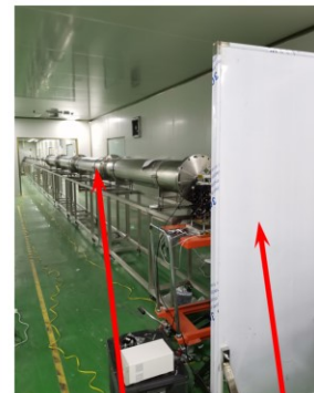
X-ray beam tube Shielding lead screen
